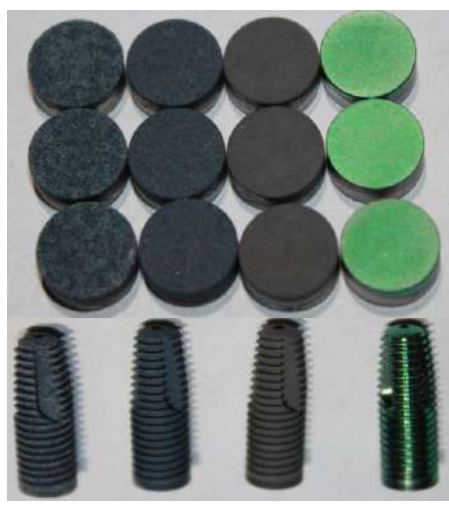
Macro view of GumMetal samples after PEO process
